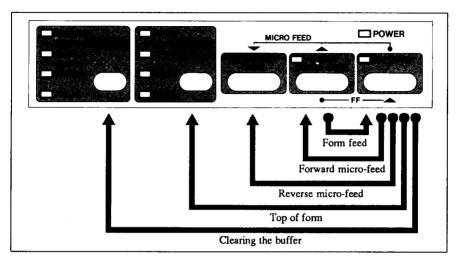
Figure 2-6. Switch combination functions of control panel
