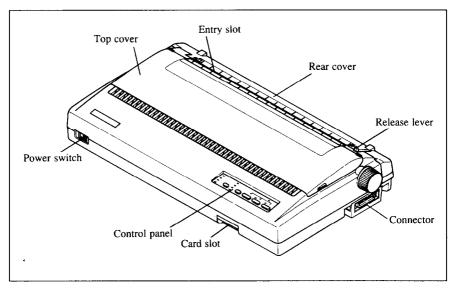
Figure 1-2. The printer's external parts
