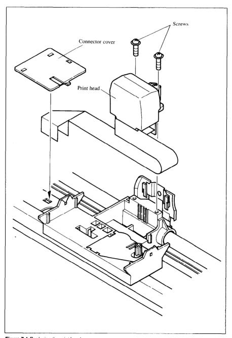
Figure 7-4. Replacing the print head
