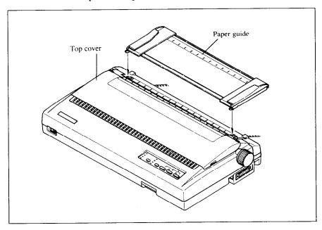
Figure 1-14. Mounting the paper guide for fanfold forms
