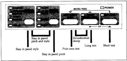
Figure 2-2. Power-up functions of control panel
