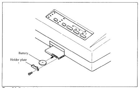
Figure 7-5. Replacing the battery.
