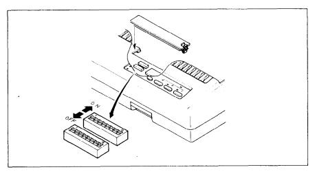
Figure 3-1. DIP switches
