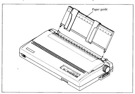
Figure 1-10. Mounting the paper guide for single sheets
