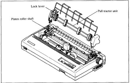
Figure 1-15. Mounting the optional pull tractor unit
