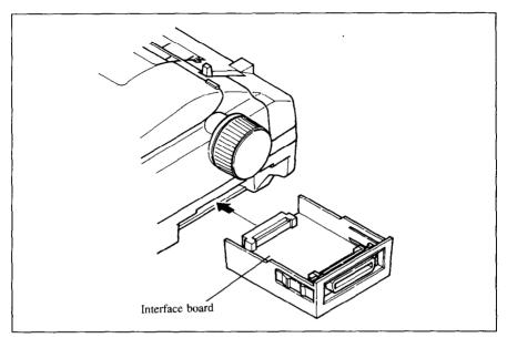
Figure 1-9. Replacing the interface board
