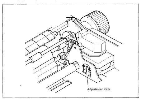
Figure 1-16. Adjusting for different thicknesses of paper
