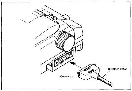
Figure 1-8. Connecting the interface cable
