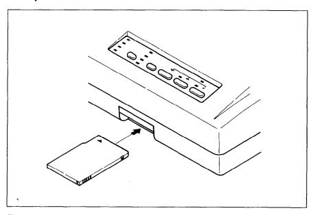
Figure 1-7. Slide the IC card into the front slot with the power switch off.
