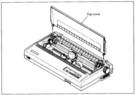
Figure 1-4. Removing the top cover
