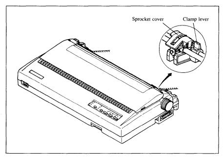
Figure 1-13. Thread the fanfold paper over the sprockets.
