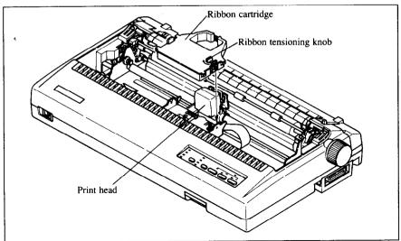
Figure 1-5. Installing the ribbon cartridge
