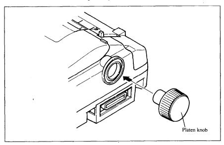
Figure 1-3. Mounting the platen knob
